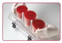
Place inoculated BD BBL™ plates in the BD GasPak EZ Petri dish rack and lower rack into BD GasPak EZ Incubation Container.
