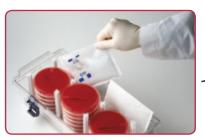
Remove appropriate number of BD GasPak EZ Gas Generating Sachets and place in container. (Use one BD BBL Anaerobe Sachet with Indicator when using the BD GasPak EZ Anaerobic System.)
