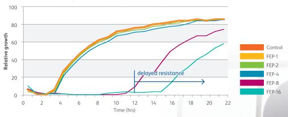
Foundation for detection of emerging resistance is not available in other automated systems: Panel design and dual technology ensure broadest antimicrobial testing, with a minimum of 3 doubling dilutions enabling detection of delayed resistance.
